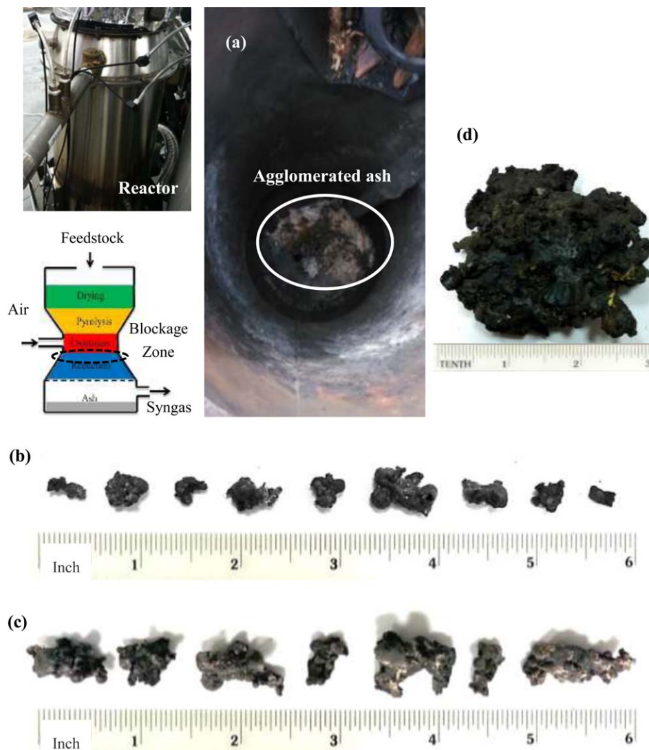
Figure 7. (a) Reactor blockage caused by the agglomeration of ash particles in the reduction zone of gasifier and the agglomerated ash particles found inside gasifier from cogasification of sewage sludge and wood chips at different sewage sludge and wood chips compositions: (b) 10 wt %, (c) 20 wt %, and (d) 33 wt % of the dried sewage sludge, respectively.
